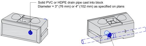
Pipe to extend 6" (152 mm) to 8" (203 mm) from back of block for connection to perforated wall drain
