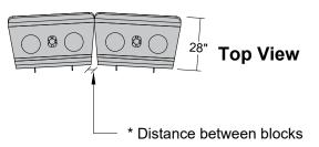
\* Distance between blocks is measured at the back of 28" (710 mm) blocks and 24" (610 mm) behind the form parting line (back edge of face texture) for 41" (1030 mm) blocks. This distance is intended to be a guide only. Minimum radius is controlling.
